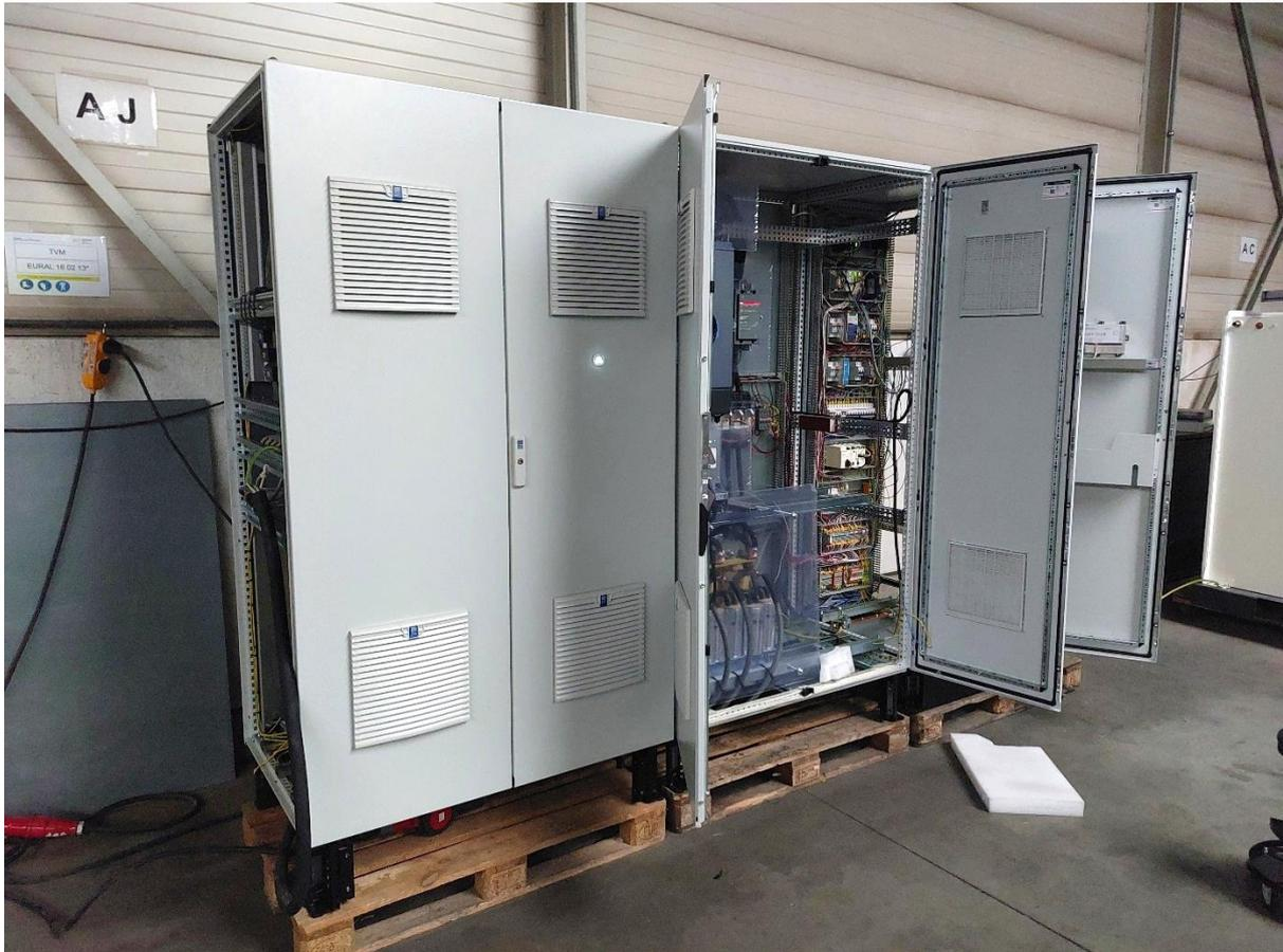
*Image 2: Power conversion cabinets under construction*
